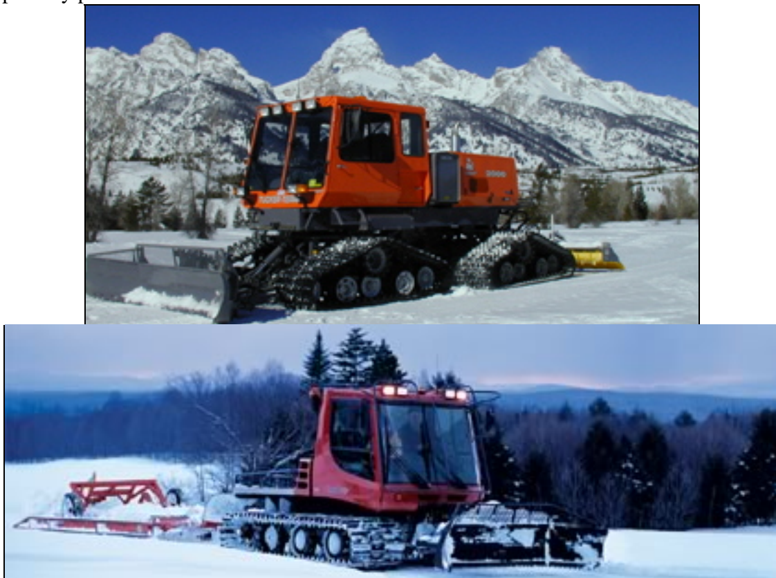
Photo 1.6 Typical specialized modern snowmobile trail grooming equipment
